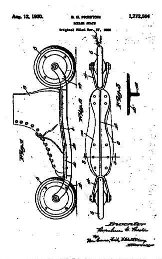
This baby, invented around 1925 by Burnham G. Preston, is another low riding inline. Designed to be riveted to a shoe, it has an "unyielding" integral frame which lies below the center of the wheels. The wheels are attached to a front and rear yoke "bicycle style". They are very large and very rubber. Truly this is another uncommon inline unlike anything we see today.
